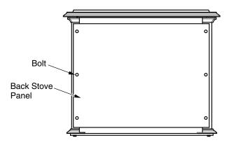
Figure 6 - Removing Back Panel (Amity Stove Only)
